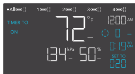
TIMER TO ON (COUNTDOWN END POINT)
